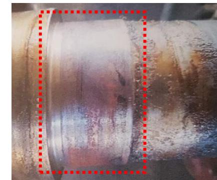
Shaft Surface Scratch (Coupling Side)
