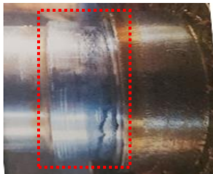
Shaft Surface Scratch (Fan Side)
