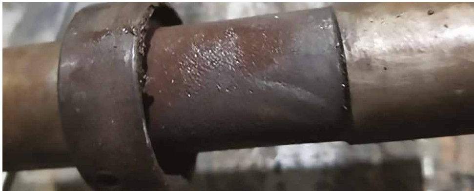
Damaged shaft from bearing failure.
