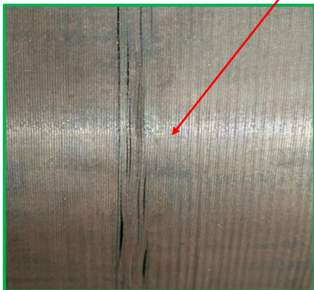
Figure 4# Rotor crack in close view
